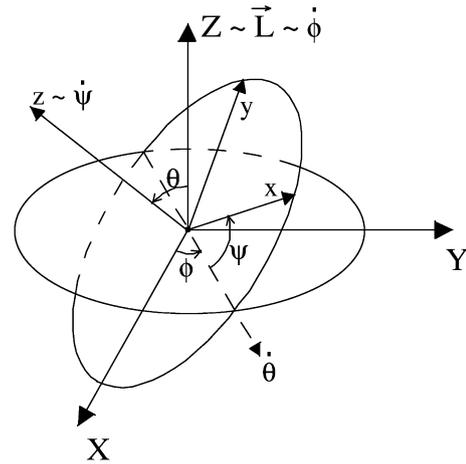
Fig. 1. Inertial reference frame  $XYZ$ , the body-frame coordinate system  $xyz$  and Euler angles  $\phi$ ,  $\psi$ ,  $\theta$  describing the orientation of the body.
